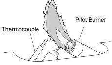
Figure 18 - Incorrect Pilot Flame Pattern
